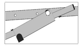
The smaller Addaline frame is raised by manually securing the wire Braces into the Side Arm's larger punched holes. To lower the frame, hold the front bar and remove each wire Brace from the Side Arm hole. Carefully lower frame.
